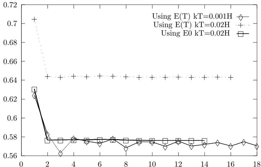
Figure 2.4: The surface energy ( $\text{J}/\text{M}^2$ ) of Li(100) for various numbers of layers in a slab model showing the effects of WIDTH (0.02H and 0.001H) and the use of E(T) or E0
