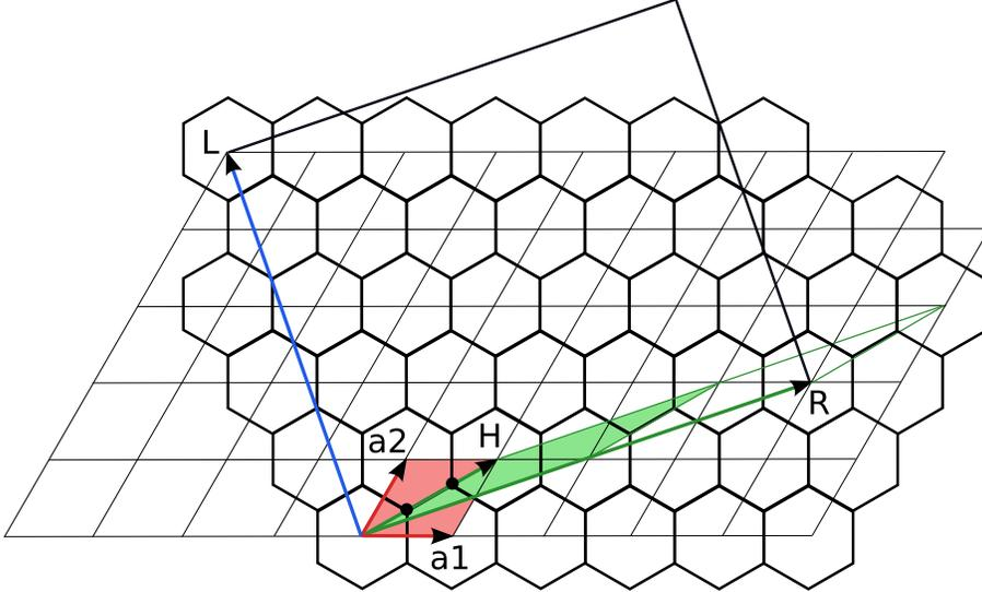
Figure 2.3: Building the (4,2) SWCNT from graphene.
